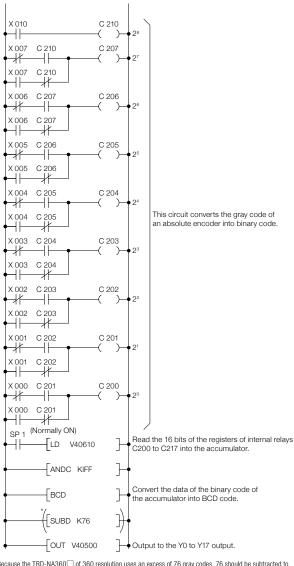
Because the TRD-NA360□ of 360 resolution uses an excess of 76 gray codes, 76 should be subtracted to make the BCD output code of 0° to 360°.
