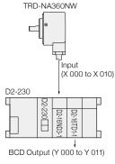
The conversion from gray code to BCD by the programmable controller is limited by the program  $% \left( 1\right) =\left( 1\right) \left( 1\right) \left$ execution processing time. Therefore, when 1 scan is 20 ms, correct data is not obtained unless the rotating speed of the encoder is not more than 8 rpm.
