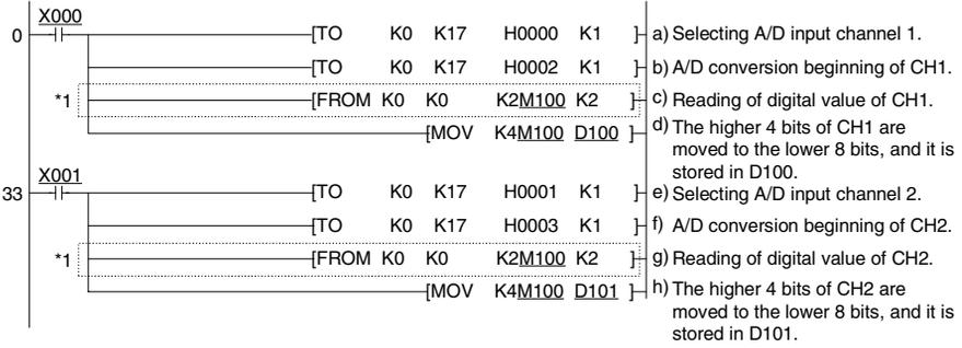
Analog to digital conversion execution input of CH1:X000
