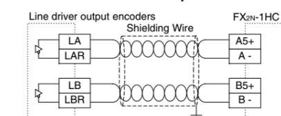
When applying the Differential-Line-Driver encoder (AM26C31 or equivalent) to FX2N-1HC, connect the encoder output with the 5V DC terminal as shown in the left figure.
