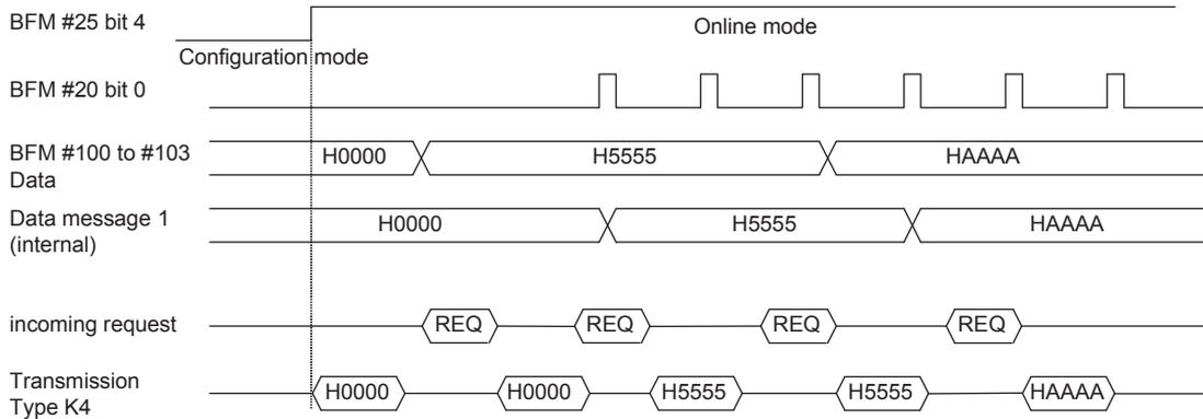
2) Transmission Type K4 (trigger via PLC/user flag)
