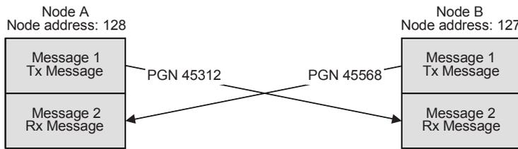
Message 1 of Node A and Node B are configured as transmit (Tx) messages. Node A uses PGN 45312 for its Tx message, Node B uses PGN 45568 for its Tx message.
