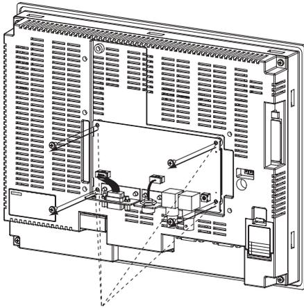
Remove the screws securing the four corners.
