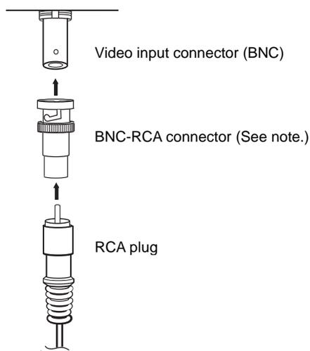
\* The BNC-RCA connector is not provided with the RGB and Video Input Unit (NS-CA002).
