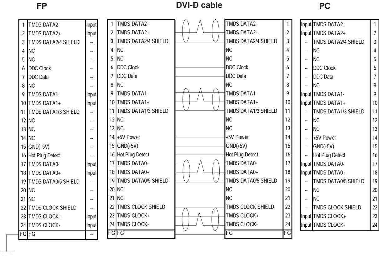
Signals and signal names used with the FP and the DVI-D cable (optional cable) are the same as those used for PCs. Also, the same pin is used on both sides of the optional cable so that you can connect the cable regardless of the cable direction.
