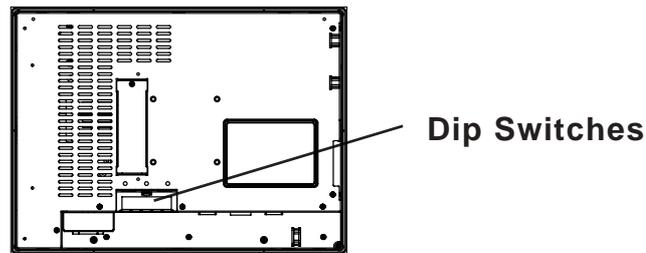
The FP unit's Dip Switches are preset as shown below. These settings are made on the assumption that a Windows® compatible computer is used.
