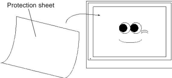
Attach the screen protection sheet when using the FP in extremely dirty or dusty areas.
