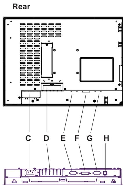
E: VGA Interface (analog RGB) Connector
