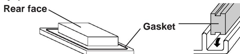
■ **Create a Panel Cut and insert the GLC into the panel from the front**
